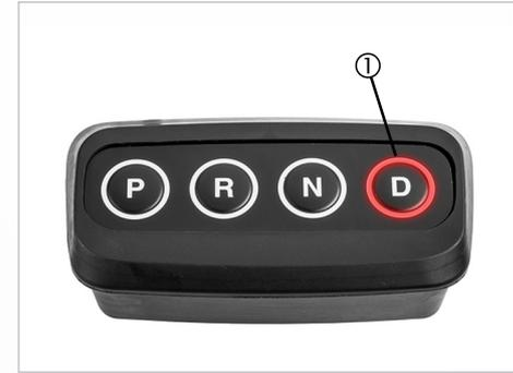
Abb. 24: Driving gear display
