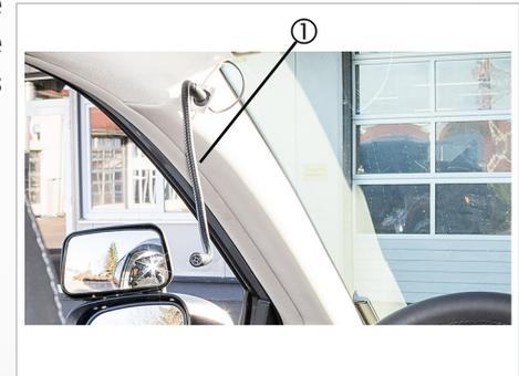
Abb. 51: Gooseneck microphone
