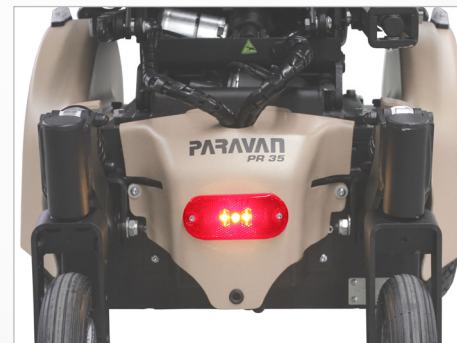
Fig. 100: Illumination at the rear
