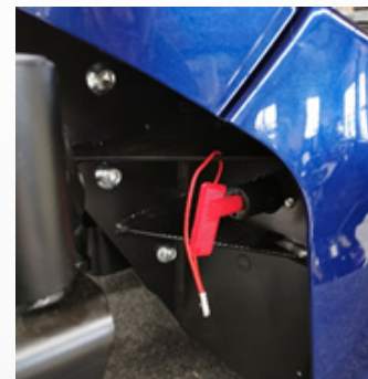
Fig. 98: Battery dicon. switch, inactive
