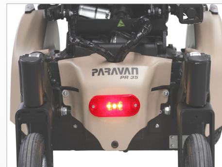
Fig. 11: Illumination at the rear
