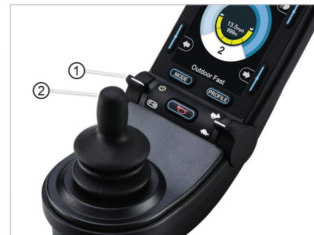
Fig. 68: Blocking the controls
