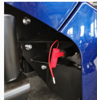
Fig. 98: Battery dicon. switch, inactive
