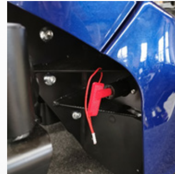
Fig. 108: Battery dicon. switch, inactive
