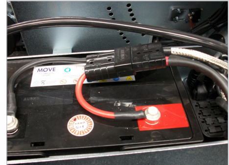
Fig. 47: Main cable battery
