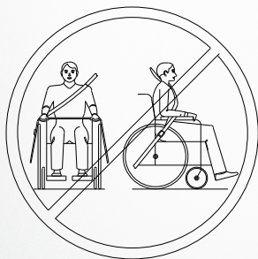
Fig. 34: Illustration of an inadequate belt system
