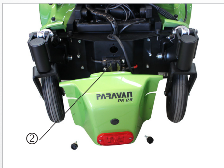
Fig. 24: Rear light, cable
