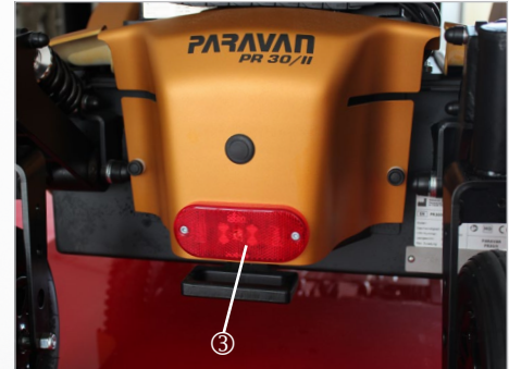
Fig. 105: Illumination at the rear
