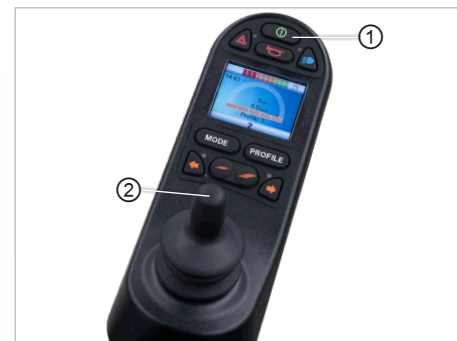
Fig. 95: Blocking the controls
