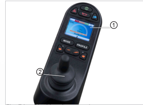
Fig. 74: Blocking the controls
